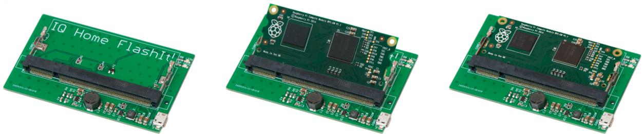
5. Connect FlashIt! to the PC with a micro USB cable
